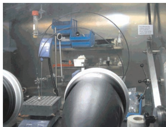
Figure 5. Setup with the ATR-IR probe inside an argon purged glove box.
