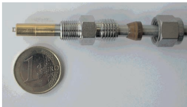
Figure 1. Fibre probe by ifs-aachen with diamond prism as internal reflection element and a 1 Euro-coin (diameter 23 mm) for size relation.
